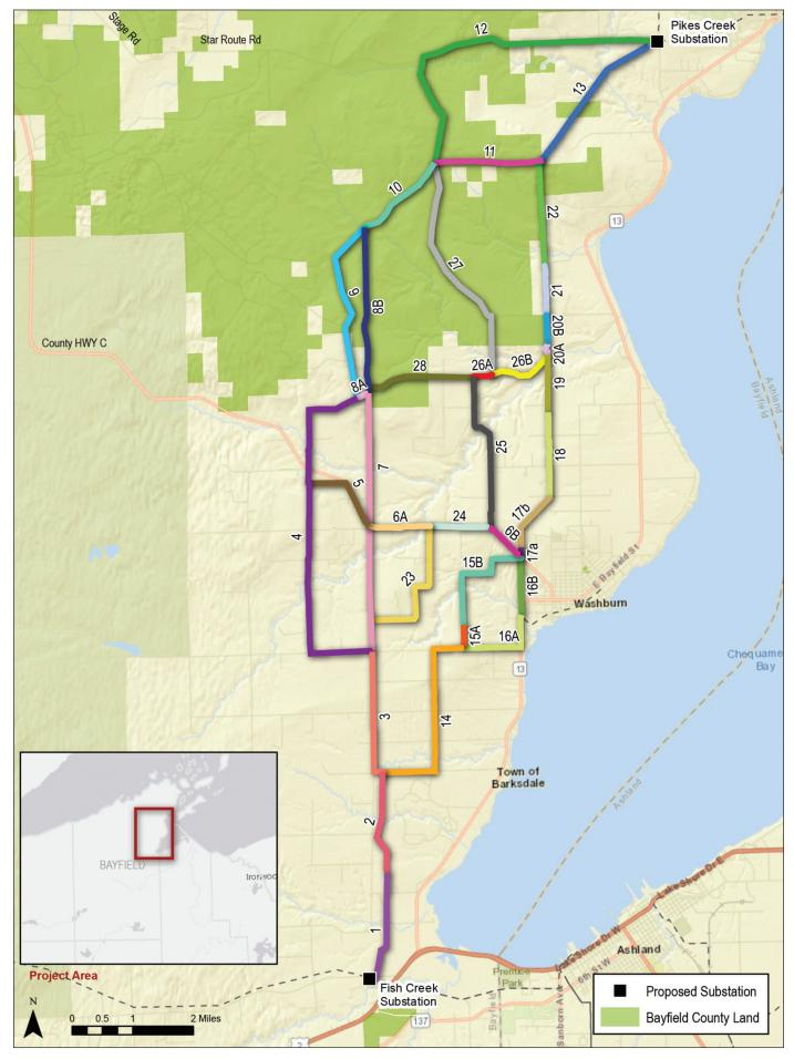
The different colored lines and corresponding numbers on the map represent all of the potential route segments currently being considered. Several combinations of individual segments are possible to connect the new Fish Creek Substation to the new Pikes Creek Substation. View an interactive map with more details on the project website at xcelenergy.com/Bayfield.
