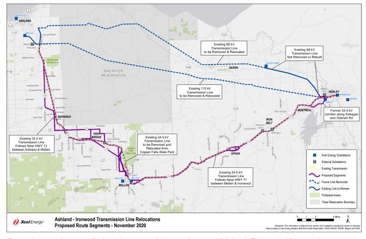
The project overview map displays the proposed route options at a high level. The colored lines on the map designate the four potential routes for the new transmission lines. Each of the four routes have a varying combination of shared route segments.
