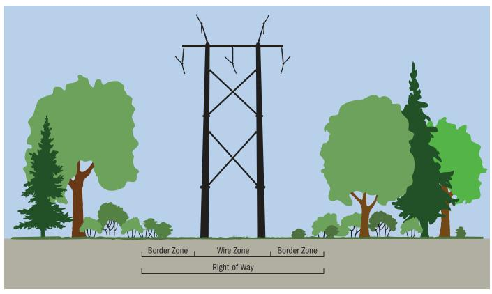
Do not plant non-compatible vegetation in the border zone or wire zone of a transmission right of way as they will likely require removal.
