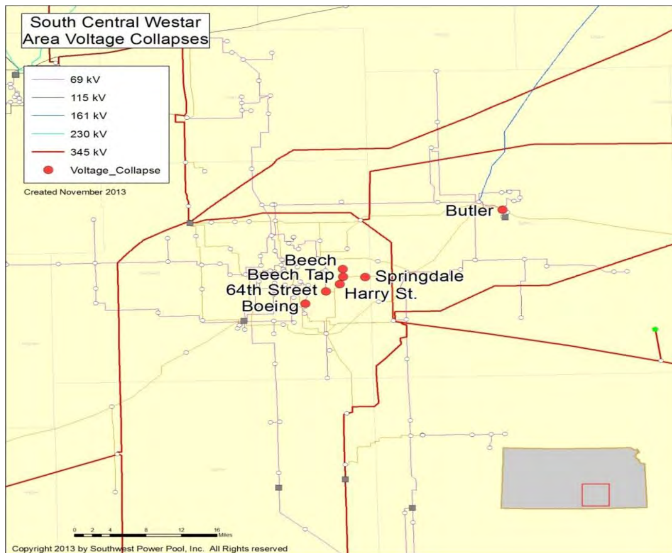
Figure 4.1: Wichita Load Area Buses Experiencing Voltage Collapse
